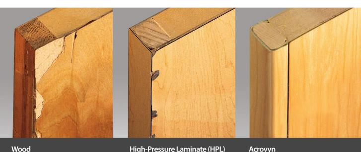
In a real-world impact test, Acrovyn Door's edge durability doubled that of wood and high-pressure laminate.
