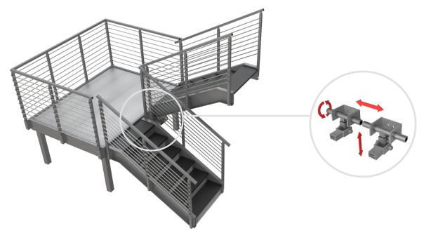
DriftReady Stairs move with the building, so instead of acting like a brace and transferring damaging forces back to the building, the system flexes and accommodates the movement without impacting the stair connection or the surrounding structure. Typical stairs with fixed connections, bolted or welded, inadvertently create a rigid column which can disrupt how the structure was engineered to accommodate seismic movement and interstory drift.
