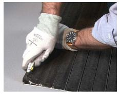
**6** For proper fit, the end trim can be cut in any of the grooves that are spaced 1/8" apart using a sharp utility knife. Score several times to cut
