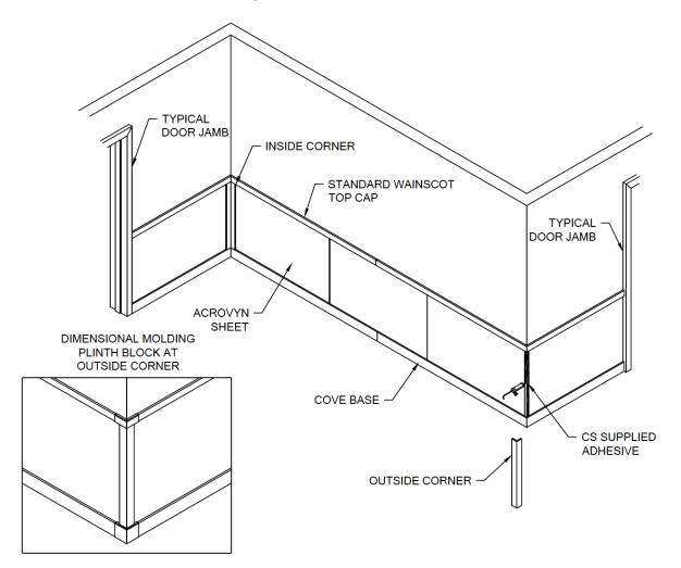
Step 11: Inside and Outside Vertical Corner Installation
