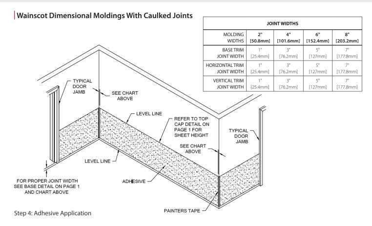
Use the 1/8" [3.175 mm] v-notch trowel to apply Acrovyn interiors heavy duty water based mastic adhesive to an area of the wall surface that can be completed within the cure time of the adhesive. Make sure the entire area receives an even coat.
