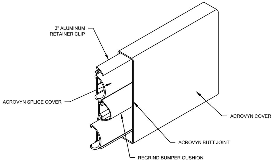
**NOTE:** INSTALLATION OF LINEAL OR RADIAL SCR-48N CRASH RAIL SHOULD BE DONE IN ACCORDANCE WITH THE FOLLOWING INSTRUCTIONS.
