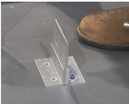
**11** Place one vertical support bar against one of the installed angled leg clips. Place another angled leg clip, facing the opposite direction of the already installed angled leg clip and vertical support bar, creating an upside down T shape and sandwiching the vertical support bar.
