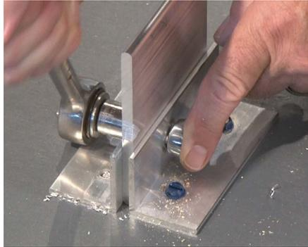
**15** Use a 1/2" socket/wrench and the supplied nut/bolt hardware to fasten all three materials together.
