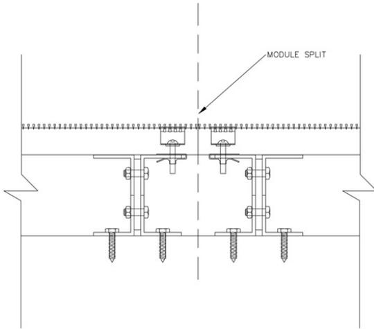
**7** Two intermediary supports will need to be installed on each side of the module split location.
