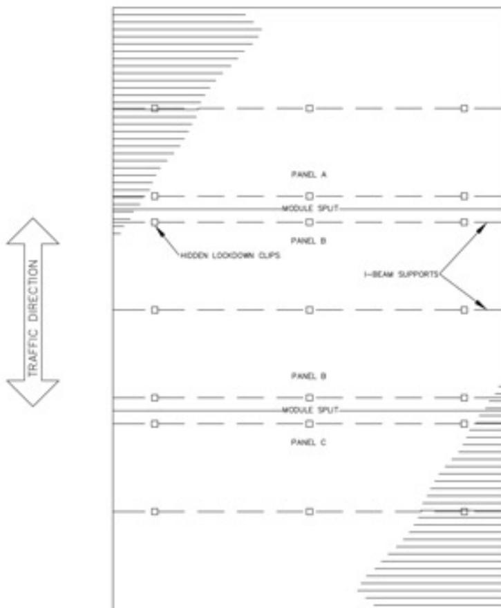
**6** Use a tape measure to locate and mark all intermediary support locations in the recess. Support locations will be at all grid module splits and every 18" on center in between the module splits. Module splits are shown on the supplied shop drawings.
