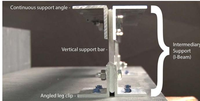
**5** These supports are comprised of a series of continuous support angles and smaller angled leg clips that need to be assembled into a finished support system. They should be installed every 18" on center.
