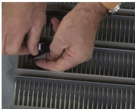
**29** Mount the screw into the welded tab. Use electrical tape to hold the screw in place.
