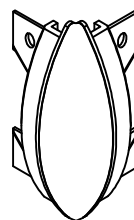
CRASH RAIL OUTSIDE CORNER ASSEMBLY
