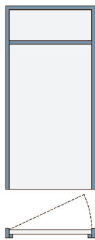
SASD+OP Single-acting single doorset with overpanel Overpanels can be glazed or unglazed
