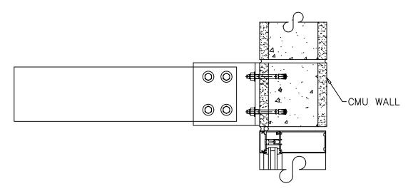
SECTION VIEW DETAIL OF CUSTOM CANTILEVER AIRFOIL SUNSHADE SYSTEM
