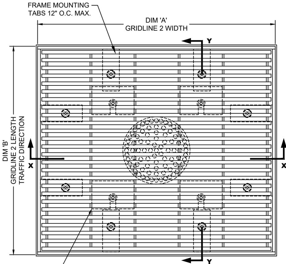
1/8" X 1-7/8" X 1-1/4" HOLD-DOWN PLATE 1 AT EACH CORNER THEN SPACE 30" O.C. SLOT SHOULD RUN PARALLEL TO SUPPORTS ALL FACING SAME DIRECTION (90F040001).
