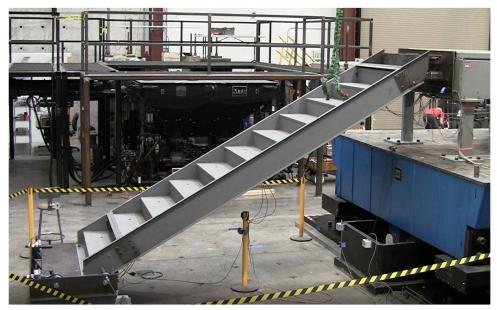
Figure 2.1 Testing Machine with Stair System Installed
