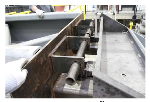
Figure 2.5 View of Upper Connection of the DriftReady<sup>™</sup> Stair System Tested
