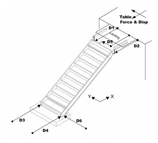
Figure 2.2 Testing Machine with Stair Specimen Installed
