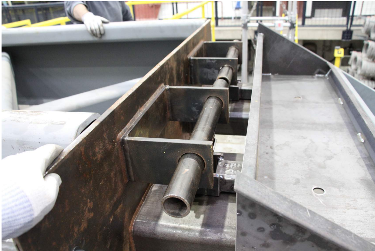
Figure 2.5 View of Upper Connection of the DriftReady™ Stair System Tested
