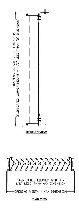
NOTE: ALL LOUVERS, PERIMETER ATTACHMENTS, AND FASTENERS TO BE DESIGNED ON A JOB BY JOB BASIS BASED ON BLAST REQUIREMENTS (LOAD [psi] AND IMPULSE [psi-msec])
