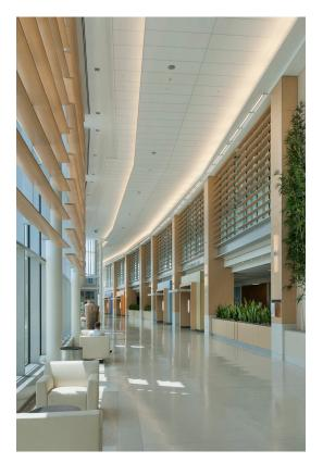
Inside the expansive atrium is filled with natural light from windows that span the length of the building. C/S Wood Wrapped Airfoils, a new interior shade product, are positioned strategically in front of the windows to help regulate and diffuse the sunlight. Used in conjunction with screening attached to the exterior curtain wall reduces the energy required to heat and cool the facility. The same shades are used as an aesthetic feature in other interior areas.
