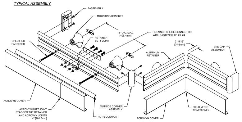
NOTE: INSTALLATION OF LINEAL OR RADIAL ECR-40N CRASH RAIL SHOULD BE DONE IN ACCORDANCE WITH THE FOLLOWING INSTRUCTIONS.
