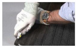
8. For proper overall fit, adjust the end trim using a utility knife with a new, sharp blade. Remove excess trim equally at both ends. The end trim has grooves every 1/8" that you can use to run the blade across.
