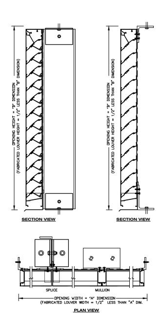
NOTE: ALL LOUVERS, PERIMETER ATTACHMENTS, AND FASTENERS TO BE DESIGNED ON A JOB BY JOB BASIS BASED ON BLAST REQUIREMENTS (LOAD [psi] AND IMPULSE [psi-msec])
