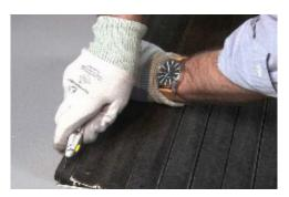
12. For proper overall fit, adjust the end trim using a utility knife with a new, sharp blade. Remove excess trim equally at both ends. The end trim has grooves every 1/8" that you can use to run the blade across.
