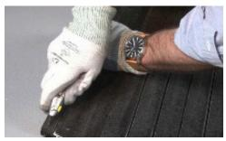
5. For proper overall fit, adjust the end trim using a utility knife with a new, sharp blade. Remove excess trim equally at both ends. The end trim has grooves every %" that you can use to run the blade across.
