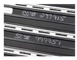
1. For layout sequence of the mat units with multiple sections, refer to the shop drawings and the mark numbers placed on the backside of the mats. \*If your Pedimat system was shipped in flat sections, refer to the supplemental instructions on the last page.
