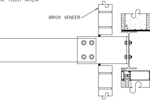
SECTION VIEW DETAIL OF CUSTOM CANTILEVER AIRFOIL SUNSHADE SYSTEM
