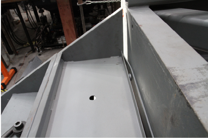
Figure 14: Yielded Mounting Plate
