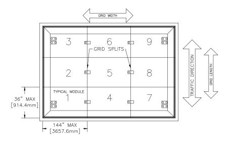
TRIAL FIT ASSEMBLY INTO FRAME AREA - TRIM END VINYL AS REQUIRED WITH A UTILITY KNIFE FOR PROPER FIT. ALIGN AND SECURE CENTER TREAD RAIL WITH LOCATOR BAR.
