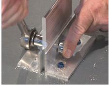
**18** .Use a 1/2" socket/wrench and the supplied nut/bold hardware to fasten all three materials together.
