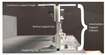
**8** These supports are comprised of a series of continuous support angles and smaller angled leg clips that need to be assembled into a finished support system. They should be installed every 24" on center.
