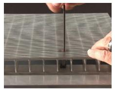
**31** Be sure all screws are properly seated into the corresponding Tinnerman clips. Repeat these steps for all grid modules.
