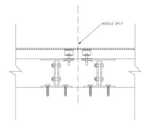
**10** Two intermediary supports will need to be installed on each side of the module split location, as shown above.
