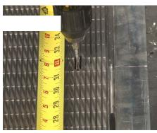
**24** Using a drill or center punch tool, transfer the marked lockdown location to the I-Beam support.
