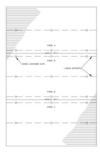
**9** Use a tape measure to locate and mark all intermediary support locations in the recess. Support locations will be at all grid module splits and every 18" on center in between the module splits. Module splits are shown on the supplied shop drawings.
