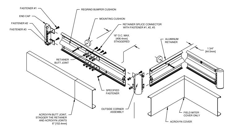
NOTE: INSTALLATION OF LINEAL OR RADIAL BCR-48N CRASH RAIL SHOULD BE DONE IN ACCORDANCE WITH THE FOLLOWING INSTRUCTIONS.
