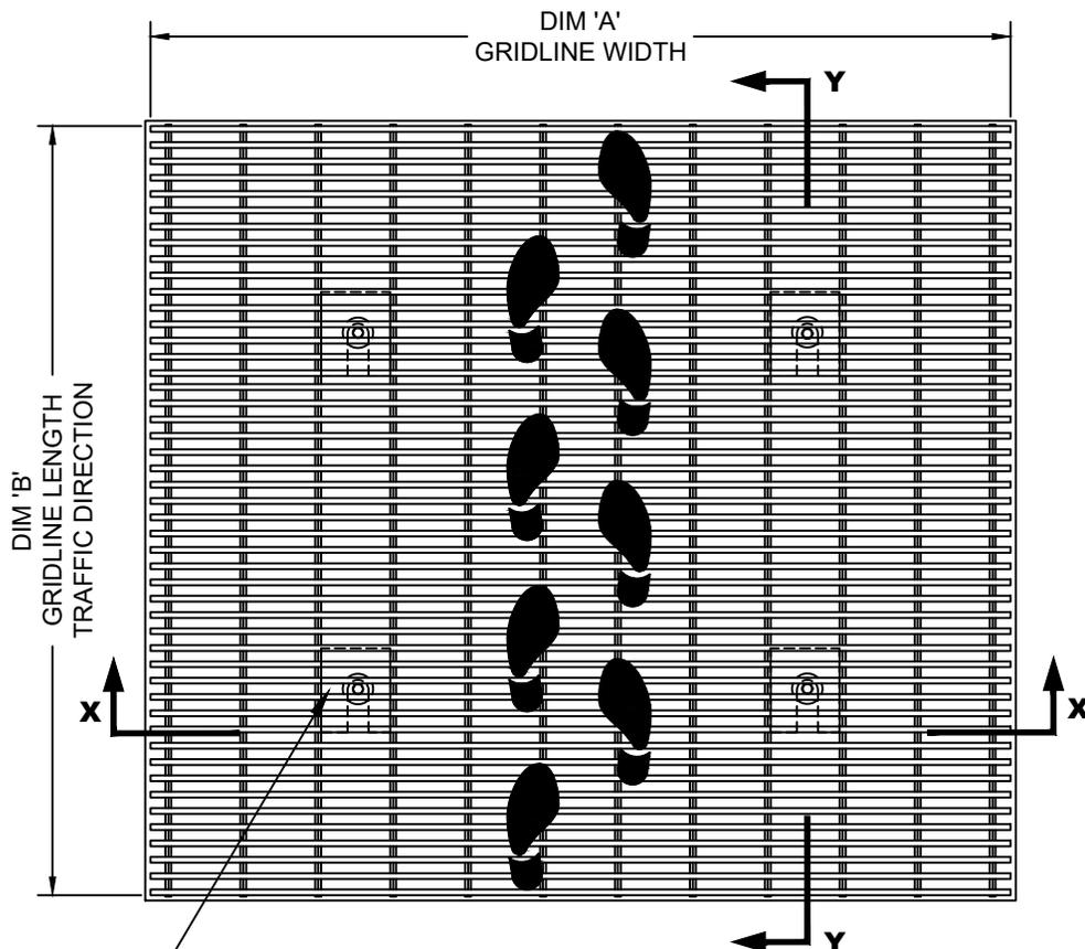
.090" X 3/4" X 15/16" SLOTTED HOLD-DOWN PLATE 1 AT EACH CORNER THEN SPACE 24" TO 30" O.C. ALL FACING THE SAME DIRECTION. (90F036001)
