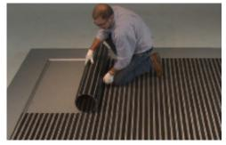
14. Care & Maintenance: to properly clean underneath the mat and avoid rail damage, roll back the mat edge to the 12th rail. Continue to roll back the mat holding that diameter.
