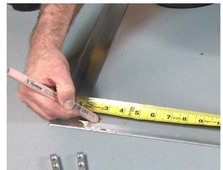
**12** Mark the center point location of the first two rails onto the frame using a carpenter's pencil.
