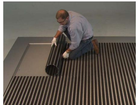
**21** Care & Maintenance: to properly clean underneath the grid and avoid rail damage, roll back the grid edge to the 12th rail. Continue to roll back the grid holding that diameter.
