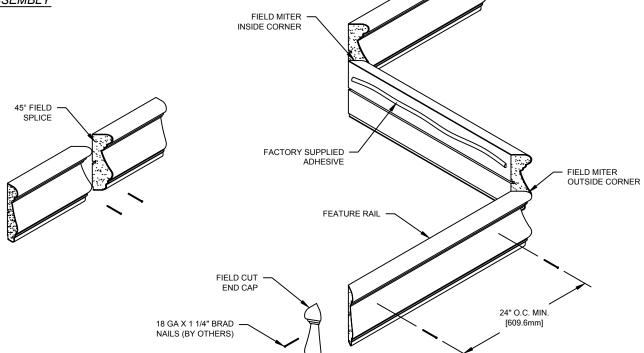
NOTE: INSTALLATION OF LINEAL OR RADIAL FR-451N FEATURE RAIL SHOULD BE DONE IN ACCORDANCE WITH THE FOLLOWING INSTRUCTIONS.
