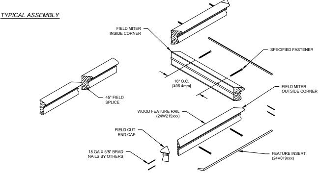
NOTE: INSTALLATION OF LINEAL OR RADIAL FRW-260 FEATURE RAIL SHOULD BE DONE IN ACCORDANCE WITH THE FOLLOWING INSTRUCTIONS.
