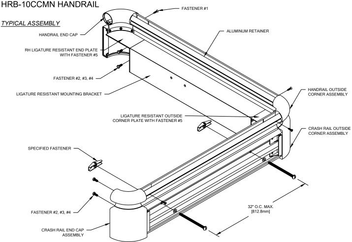
NOTE: INSTALLATION OF LINEAL HRB-10CCMN HANDRAIL SHOULD BE DONE IN ACCORDANCE WITH THE FOLLOWING INSTRUCTIONS.
