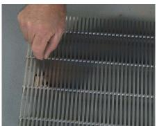
23 Beginning at the tabs in the center of the grid module, use a hex key/Allen wrench to fasten the screws into the lead shields. Continue by working your way towards the grid module edges, fastening all screws to the recess.
