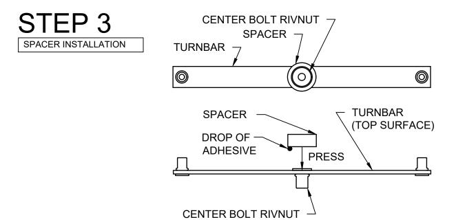
Note: A Spacer must be placed between the Turnbar and the underside (or backside) of the Cover Plate. The Spacer is used to prevent excess bowing of the Turnbars when the center bolt is tightened. (Some bowing of the Turnbars is required to apply the holding force on the Cover Plate.)
