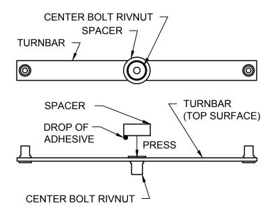
Note: A Spacer must be placed between the Turnbar and the underside (or backside) of the Cover Plate. The Spacer is used to prevent excess bowing of the Turnbars when the center bolt is tightened. (Some bowing of the Turnbars is required to apply the holding force on the Cover Plate.)
