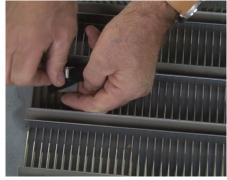
**42** For GridLine 2, mount the screw into the welded tab. Use electrical tape to hold the screw in place.
