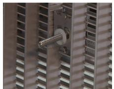
**38** Install the lockwasher onto the screw on the clip's opposite side.
