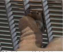
**39** Push the assembled clip into the grid so that the clip's center is aligned with the small tool.
