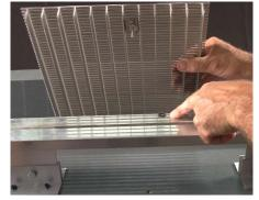
**43** For both GridLine (G6) and Grid-Line 2 (G6P), place the grid module with the installed clip/tab hardware into its corresponding Tinnerman clip location.
