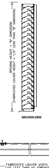
FABRICATED LOUVER WIDTH = 1/2' LESS THAN (A) DIMENSION OPENING WIDTH = (A) DIMENSION PLAN VIEW
