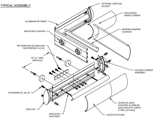
NOTE: INSTALLATION OF LINEAL OR RADIAL BCR-50N CRASH RAIL SHOULD BE DONE IN ACCORDANCE WITH THE FOLLOWING INSTRUCTIONS.
