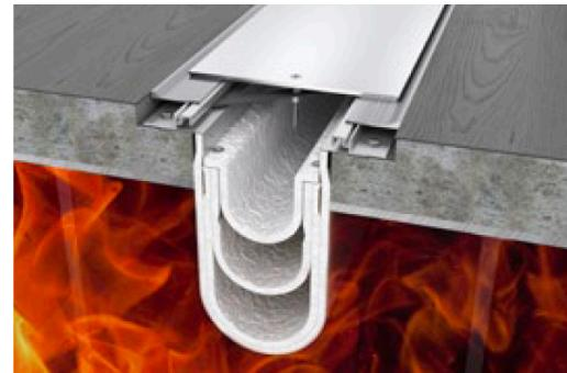
An expansion joint that runs through a building may interrupt a fire rated assembly. To maintain the integrity of the assembly and prevent the spread of fire, a tested and listed fire barrier should be incorporated.
