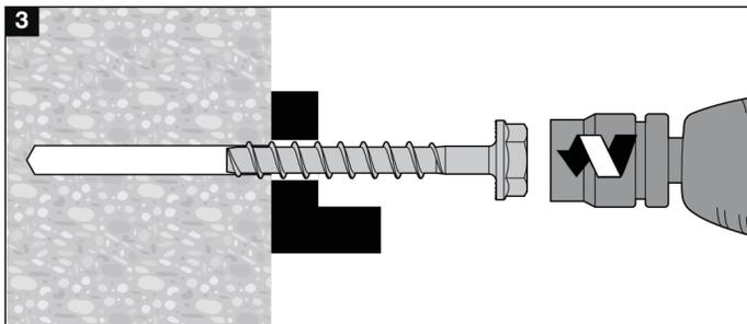
3 Fasten anchor tightly against fastened part.
