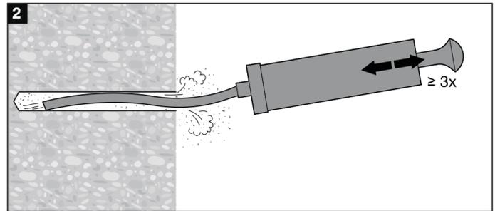
2 Clean drilled hole to remove debris.
