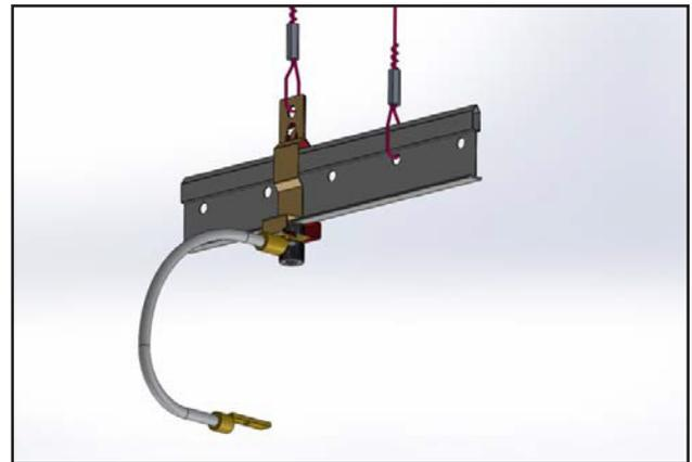
4. Attach a hanger (part# OPTS-G03N) and secure with a female OPTS-S03.
