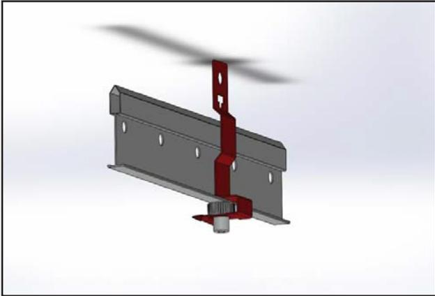
1. Insert OPTS-S03 male screw through the right clip opening of (part# OPTS-W03) and attach to ACT grid.
