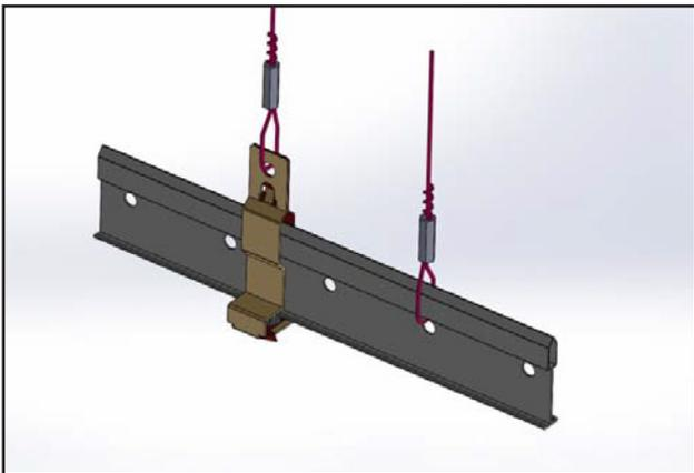
3. Secure both clips with 12 GA hanger wire up to the ceiling above.
