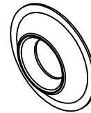
FASTENER #2 #10 COUNTERSUNK FLANGED S/S WASHER (90H047003)
