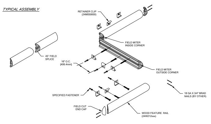
NOTE: INSTALLATION OF LINEAL OR RADIAL FRW-225 FEATURE RAIL SHOULD BE DONE IN ACCORDANCE WITH THE FOLLOWING INSTRUCTIONS.
