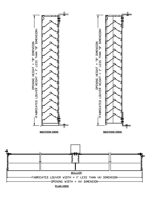
NOTE: ALL LOUVERS, PERIMETER ATTACHMENTS, AND FASTENERS TO BE DESIGNED ON A JOB BY JOB BASIS BASED ON BLAST REQUIREMENTS (LOAD [psi] AND IMPULSE [psi-msec])
