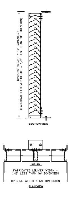
NOTE: ALL LOUVERS, PERIMETER ATTACHMENTS, AND FASTENERS TO BE DESIGNED ON A JOB BY JOB BASIS BASED ON BLAST REQUIREMENTS (LOAD [psi] AND IMPULSE [psi-msec])
