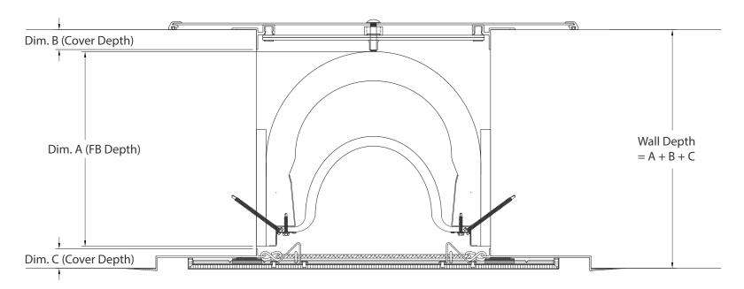
\*IMPORTANT NOTE: For wall fire barrier systems to perform properly in terms of fire rating and movement capabilities, it is important that an adequate wall depth is constructed for installation.
